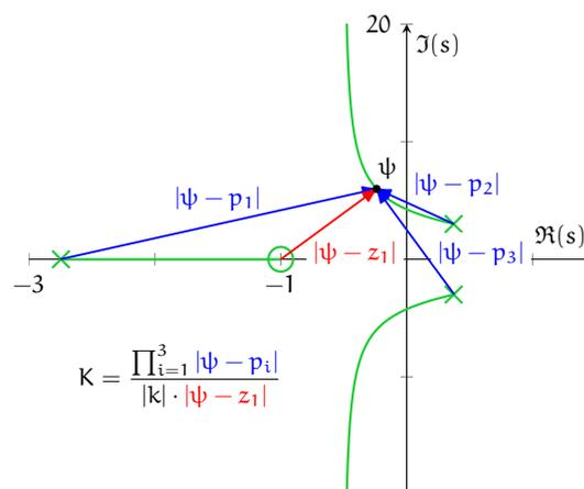
**Figure gain.1:** an example of a geometric interpretation of the the loop gain  $K$  for a closed-loop system with transfer function poles  $p_{1,2,3}$ , zero  $z_1$ , and gain  $k$  at a complex value  $s = \psi$  on the root locus.
