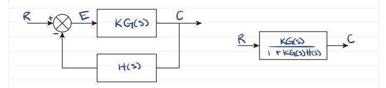
The forward transfer function is what we call KG(s). The feedback transfer function is what we call H(s). The open-loop transfer function is defined as the product of the two: KG(s)H(s).
