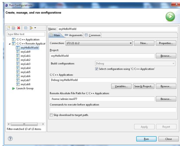
Figure 00.14: Launch Configurations.
