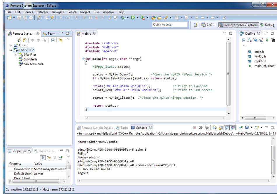
**Figure 00.12:** Remote Systems Explorer with myRIO connection successfully defined.
