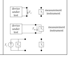
Connecting the Norton model for the device under test to the input admittance of the measurement instrument we have the network at the right.
