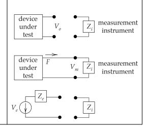
Connecting the Thevenin model for the device under test to the input impedance of the measurement instrument we have the network at the right.
