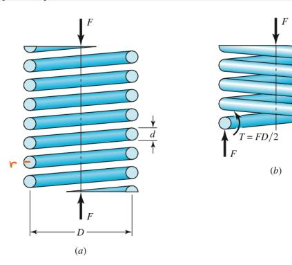
Figure 10-1b shows that the direct shear force on a given cross-section of the spring is V = F and the torsional moment T = FD/2 where D is the mean diameter. Then the torsional shear stress is maximum at the inner diameter of the spring and its value is
