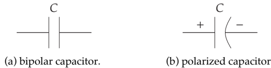
Figure 1.9. capacitor circuit diagram symbols.
