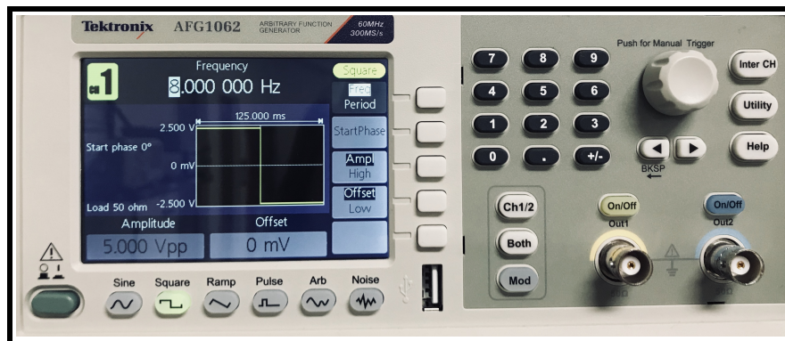
Figure 02.2: the front panel of the Tektronix AFG1062 function generator.
