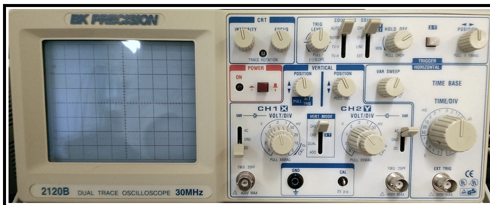
Figure 02.6: the front panel of the BK Precision 2120B oscilloscope.
