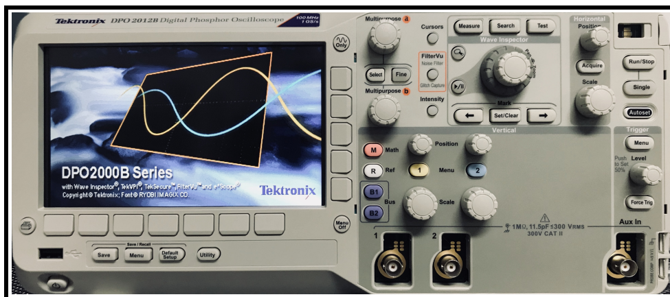
Figure 02.5: the front panel of the Tektronix DPO 2012B oscilloscope.
