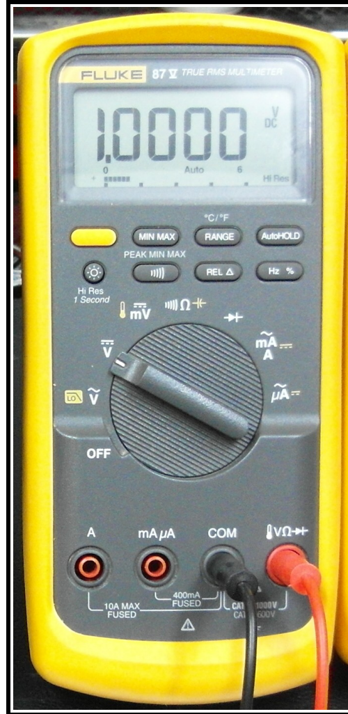
Figure 02.4: the front panel of a Fluke multimeter, connected in high-resistance mode.
