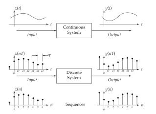
The continuous system can be described by a linear, constant-coefficient differential equation:
