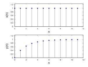
The dotted line is the exact solution y(t/T) of the original continuous differential equation. As you can see, Tustin's method is very close to the exact solution at the sample points.
